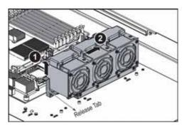
**5** Lift the fan cage (3) and unplug the connectors from it, then remove the cage from the chassis.
